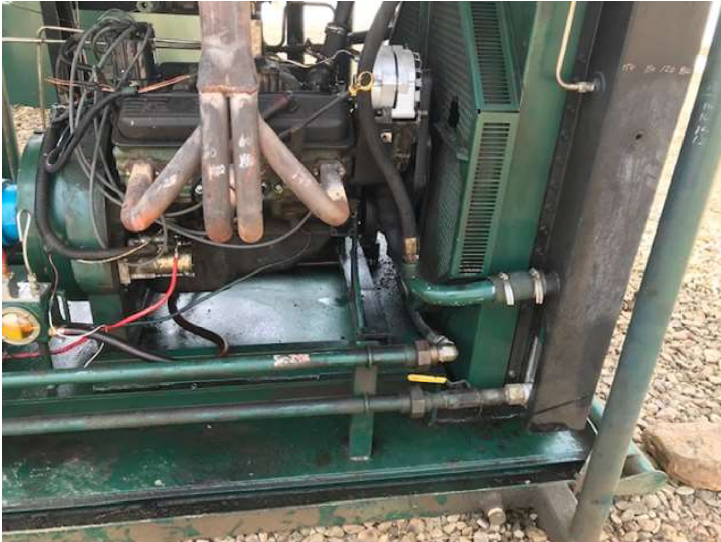
PHOTO 4: ALL VALVES AND FITTINGS WERE SECURELY FASTENED. THE SKID AND THE RESERVOIR OF THE LIQUID RING COMPRESSOR WAS CLEANED AND THE FLUID ACCUMULATION REMOVED.
