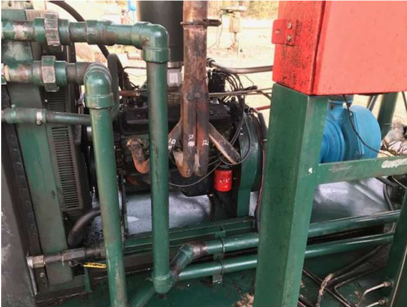
PHOTO 1: THE LEAKS FROM THE LIQUID RING COMPRESSOR WERE IDENTIFIED AND REPAIRED. THE SKID OF THE LIQUID RING COMPRESSOR WAS CLEANED AND THE FLUID ACCUMULATION REMOVED. SELF INSPECTION PROCEDURE REVIEWED BY THE SENIOR PRODUCTION FOREMAN.
