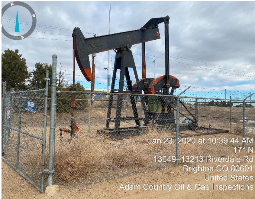
Photo#1 wellhead / Pump jack
