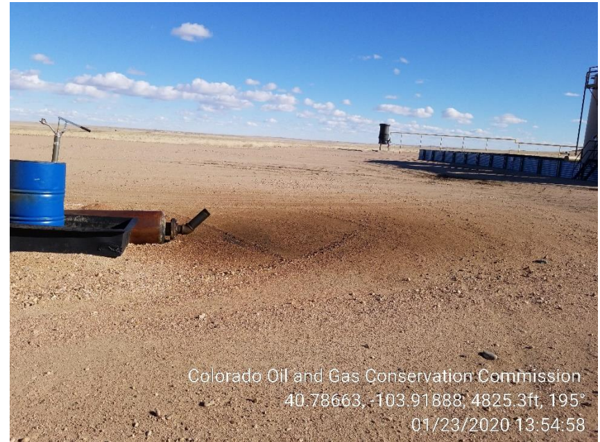
Photo 2 – Stained Soil at engine exhaust
