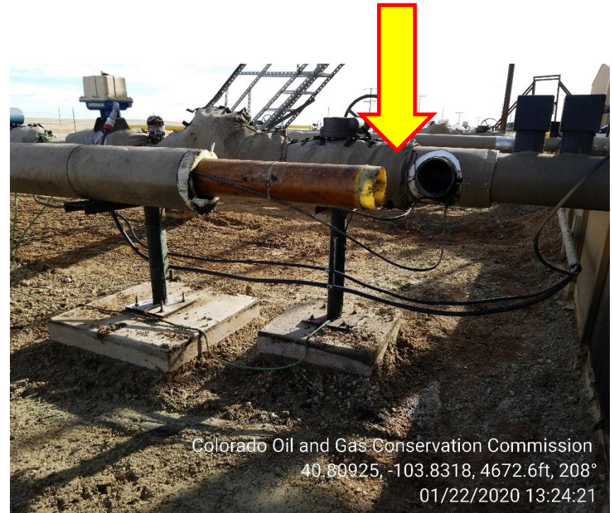
Photo 2 – 6" pipe where 90 broke
