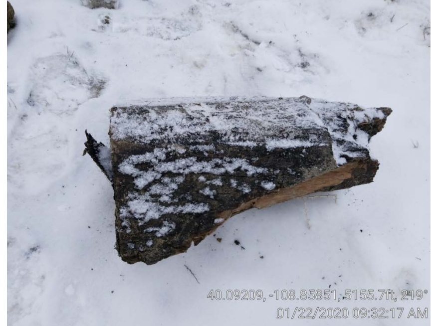
Photo 4. Wood used to plug well bore in ~1953.
