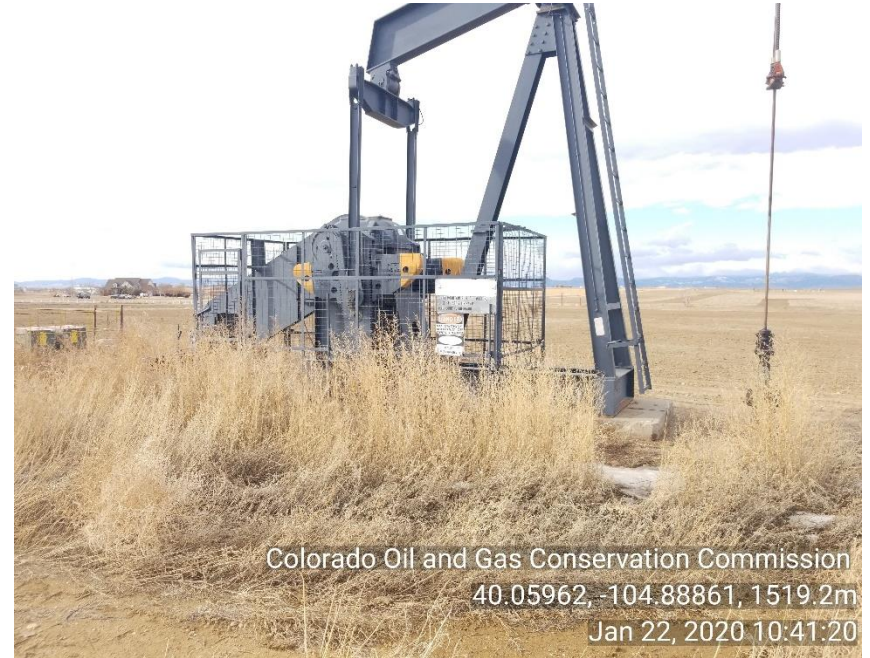
Photo 2 WH sign faded not legible, weeds around equipment
