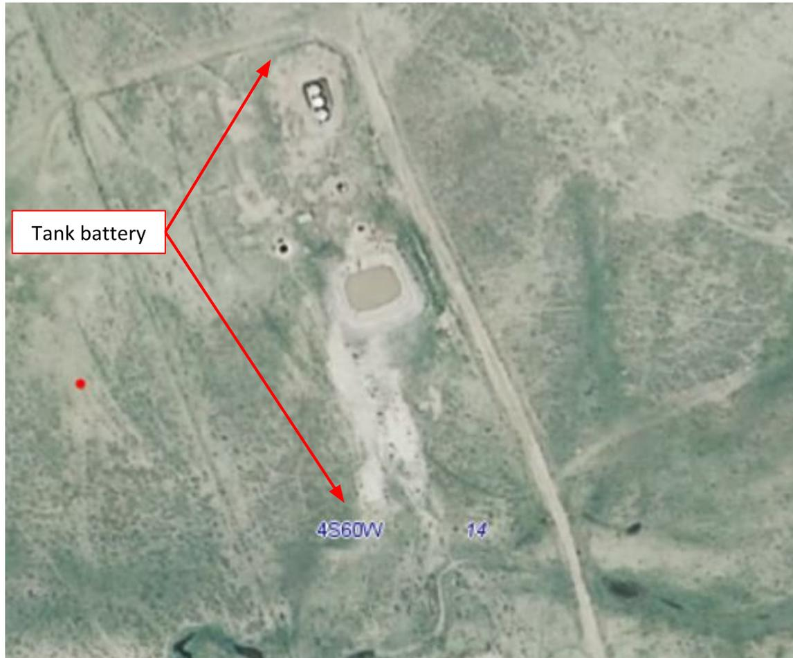
**Photo 2.** Zoomed in photo of the tank battery location. Photo illustrates the total disturbance including a produced water pit spill.
