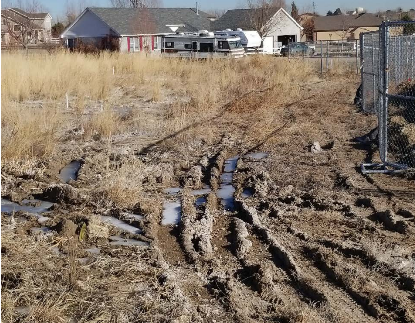
Photo 3: Wetland to the north of the perimeter fence. Some of the 16 temporary piezometers (vertical narrow white PVC pipes) are visible.
