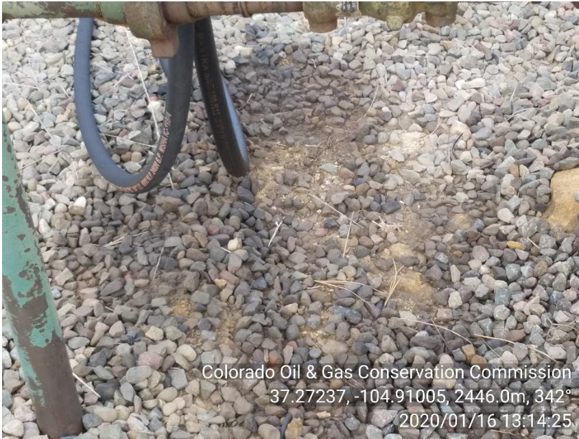
PHOTO 3: AREA OF IMPACTED SOIL NEAR WELLHEAD APPEARS TO BE COMING FROM HYDRAULIC HOSE. Non E&P Waste not properly stored, handled, transported, treated, or disposed per Rule 907A. CA DATE 2-16-20
