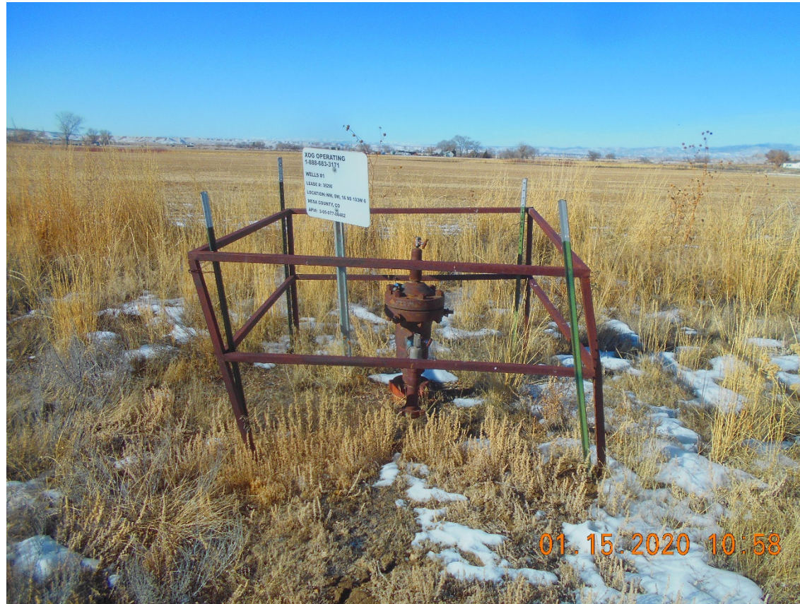
Temporarily Abandoned Wellhead
