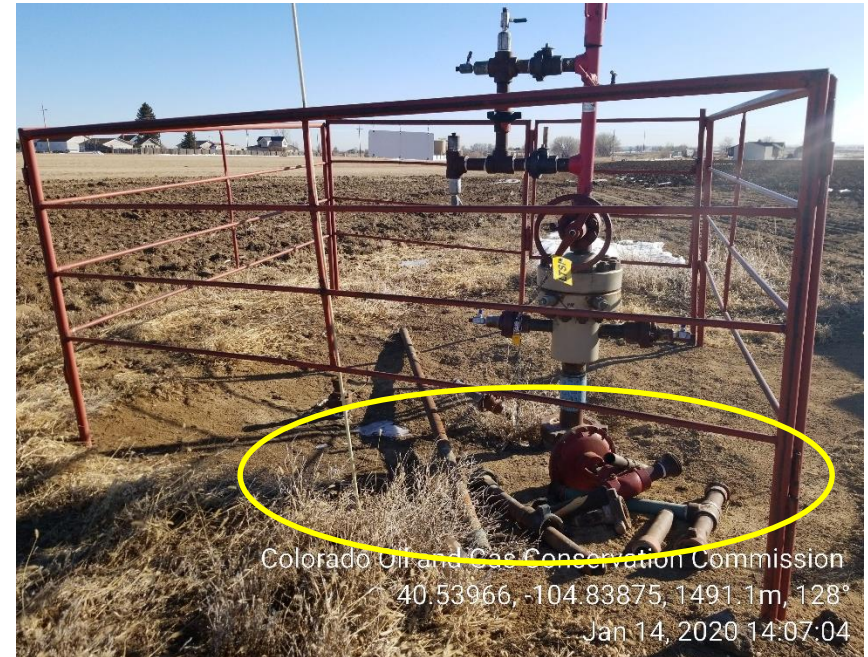
Photo 2: Wellhead; UNUSE EQUIPMENT
