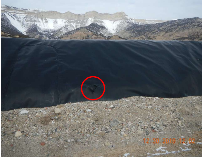
Photo #17 – 3-inch hole (Red circle) located on the southwest corner of the pit liner.
