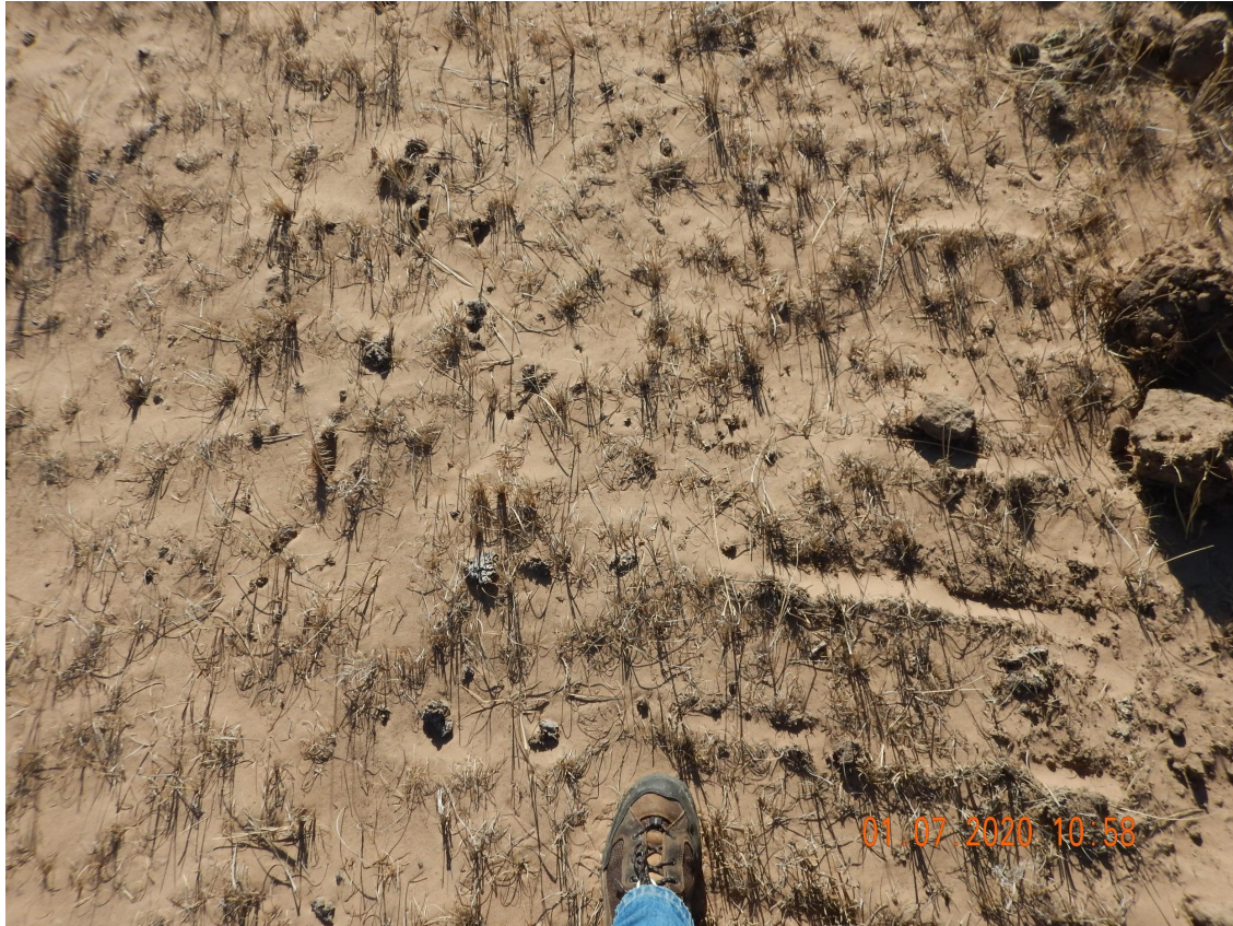
Photo 11. Close up photo taken from the eastern perimeter of location. Photo illustrates soil particle deposition accumulation outside the perimeter BMPs.
