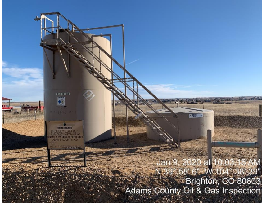
Photo #1 Crud Produced Water tanks
