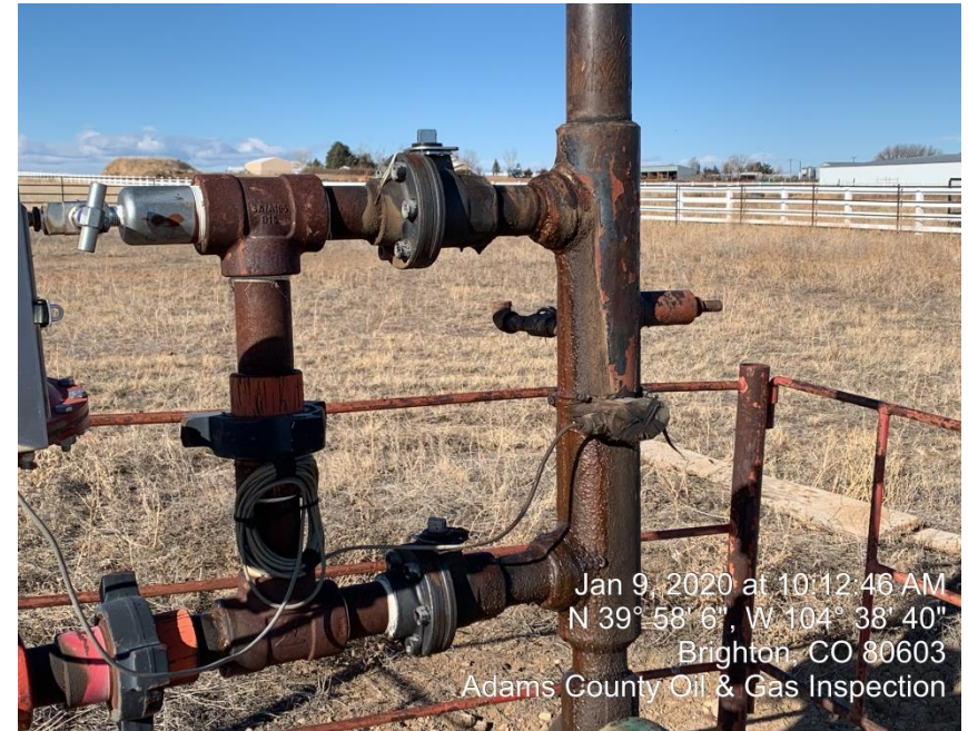
Photo#6 Lubricator leaking
