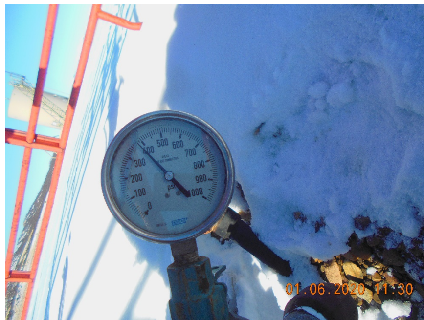
Wellhead gauge at end of test
