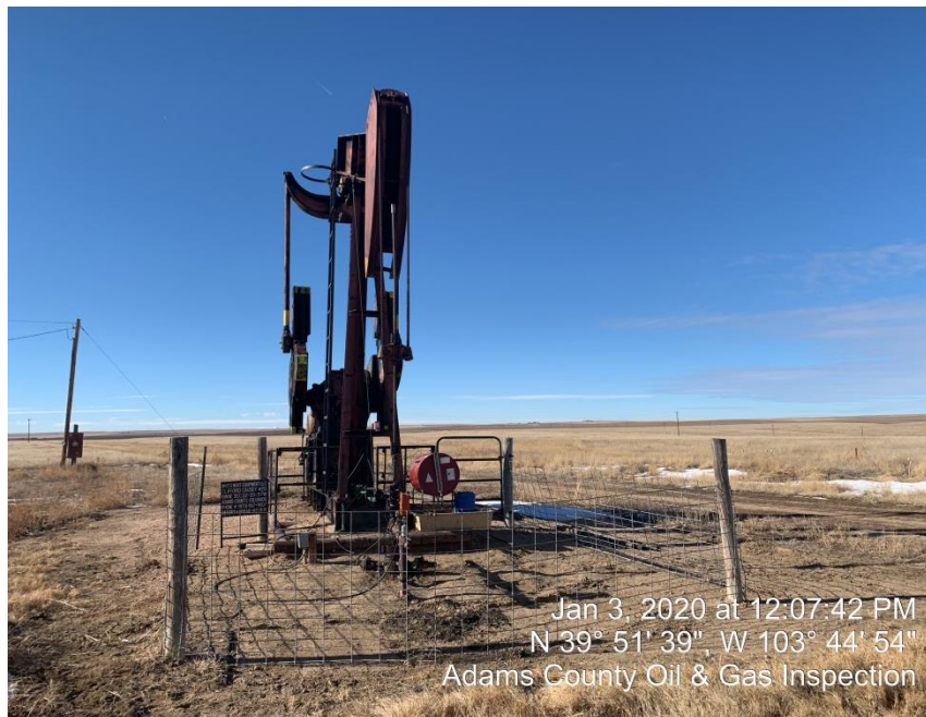
Photo#1 Pumpjack and Wellhead
