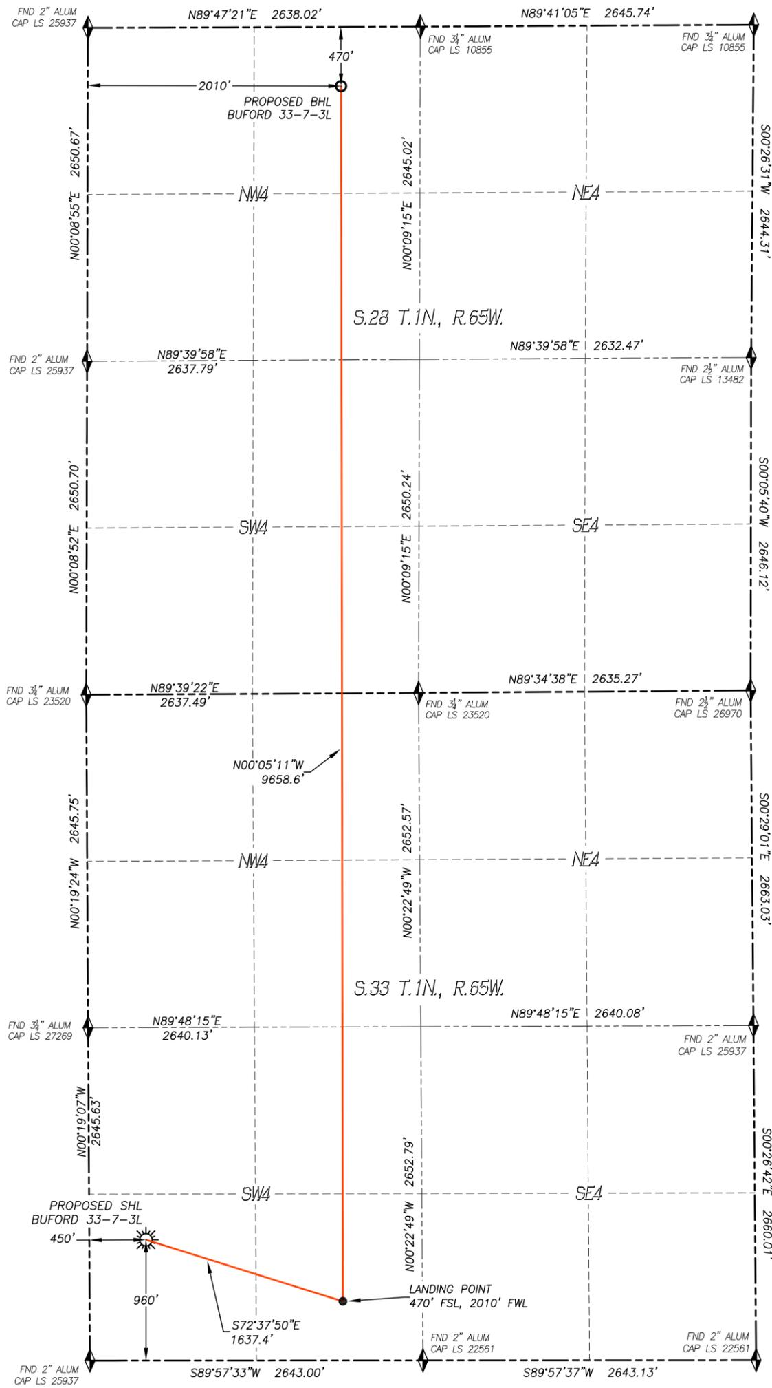
IN ACCORDANCE WITH A REQUEST FROM CONFLUENCE RESOURCES, DALEY LAND SURVEYING, INC. HAS DETERMINED THE SURFACE LOCATION OF THE BUFORD 33-7-3L WELL TO BE 960' FSL, 450' FWL, AS MEASURED AT NINETY (90) DEGREES FROM THE SECTION LINES OF SECTION 33, TOWNSHIP 1 NORTH, RANGE 65 WEST AND THE BOTTOM HOLE LOCATION TO BE 470' FNL, 2010' FWL, AS MEASURED AT NINETY (90) DEGREES FROM THE SECTION LINES OF SECTION 28, TOWNSHIP 1 NORTH, RANGE 65 WEST, OF THE 6TH PRINCIPAL MERIDIAN, WELD COUNTY, COLORADO.
