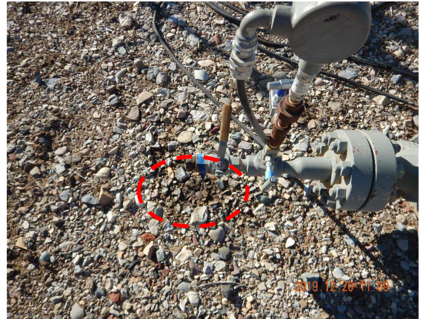
Photo #12 - Localized accumulation of oil-stained soil observed on north side of PB15 Clem Jr. 15-2BB wellhead.
