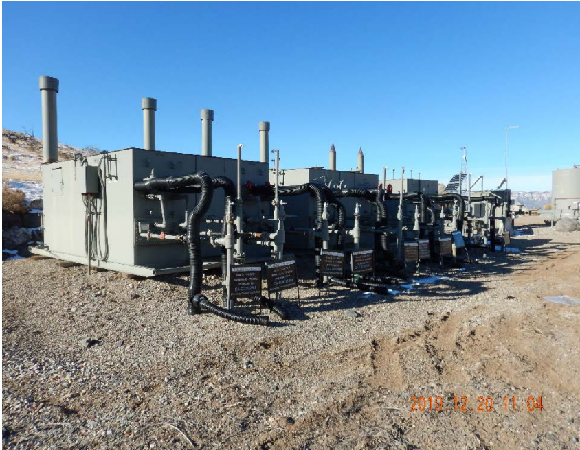
Photo #1 – View of separators on south side of pad.
