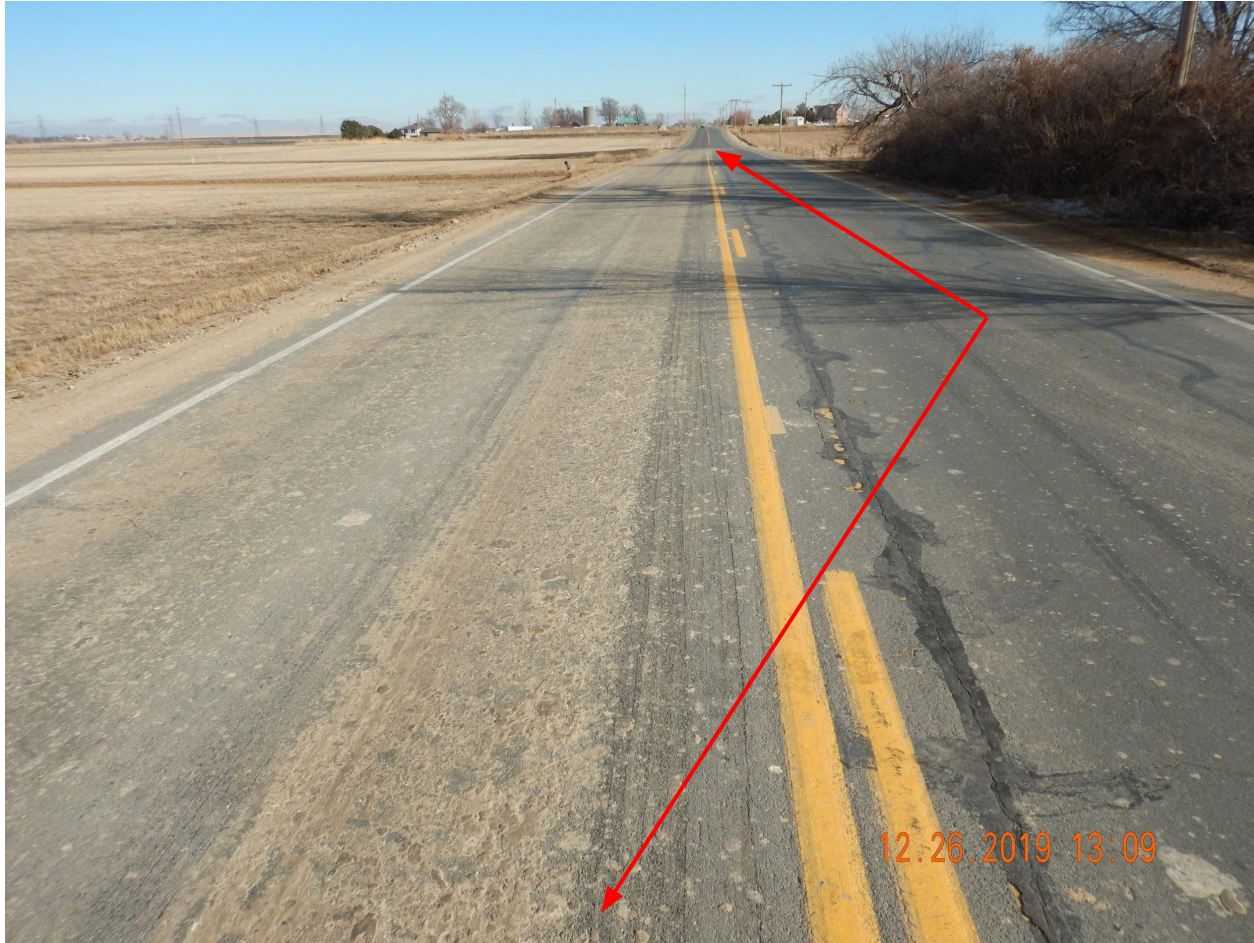
Photo 6. Photo taken ~500 feet west of the entrance on CR 2, facing East. Photo illustrates material tracked onto the county road.
