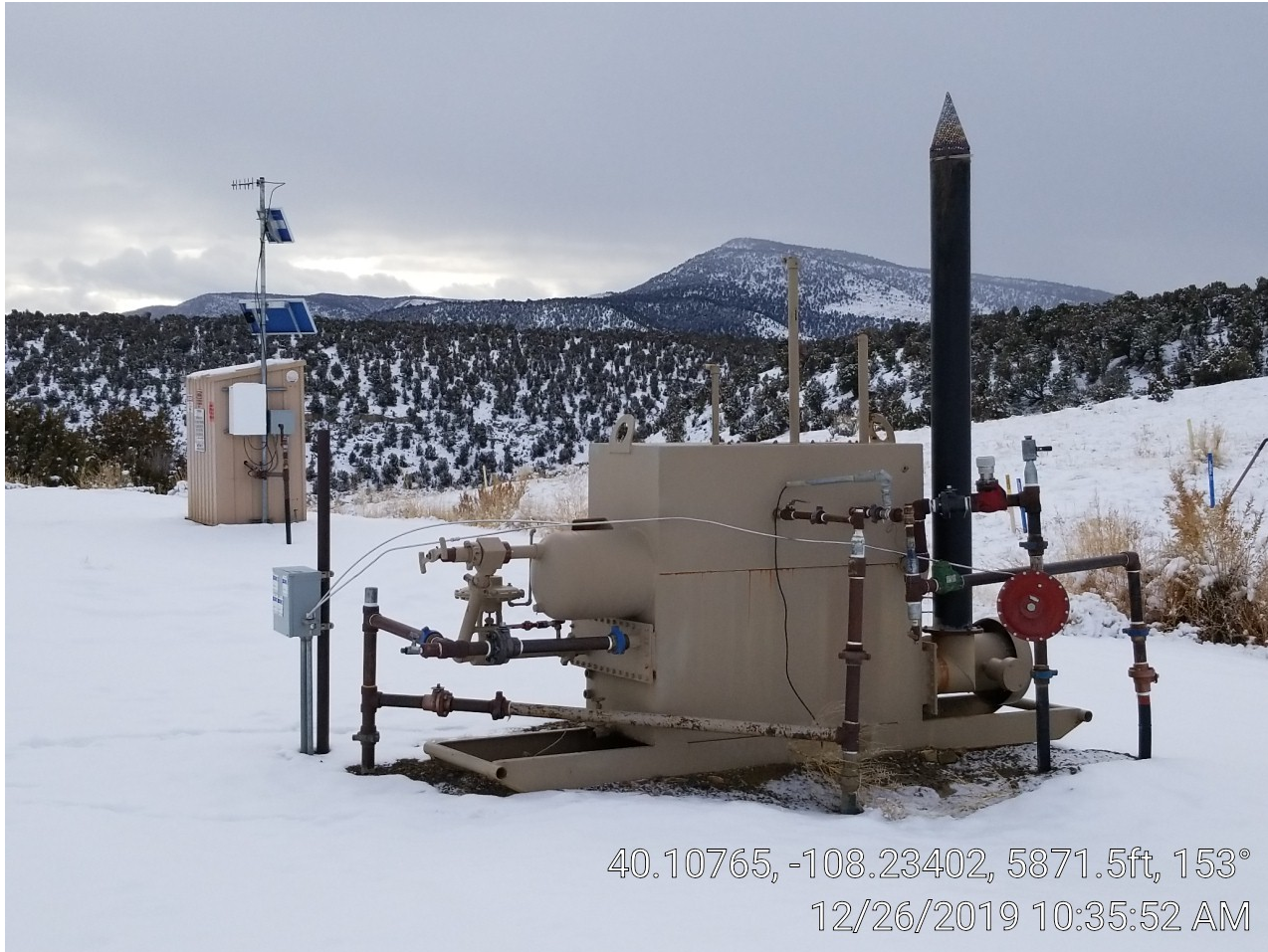
Photo 3. Meter building & separator.
