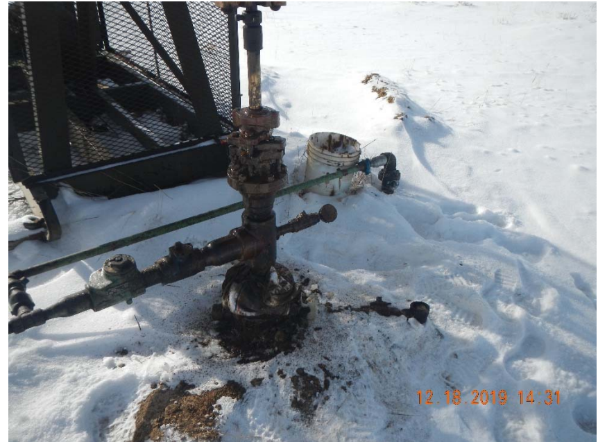
Photo 2. Stained soil at wellhead. Rags stuffed into wellhead. Bucket of oily waste without containment in right hand background of photo.
