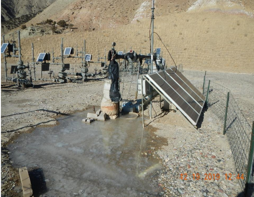
4 - batteries not properly stored sitting at injection well.
