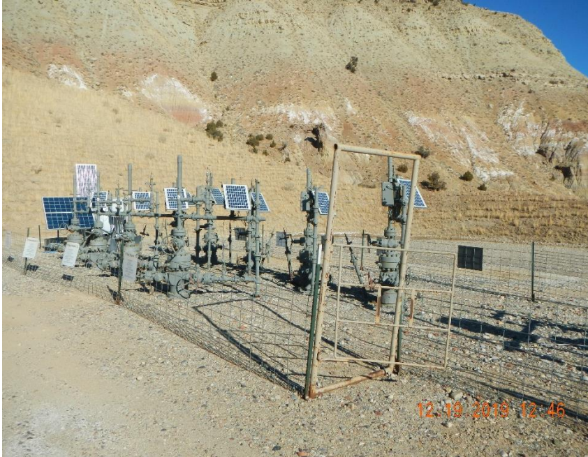
Gates on well head fencing are leaning
