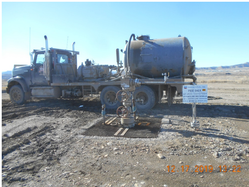
Injection wellhead.
