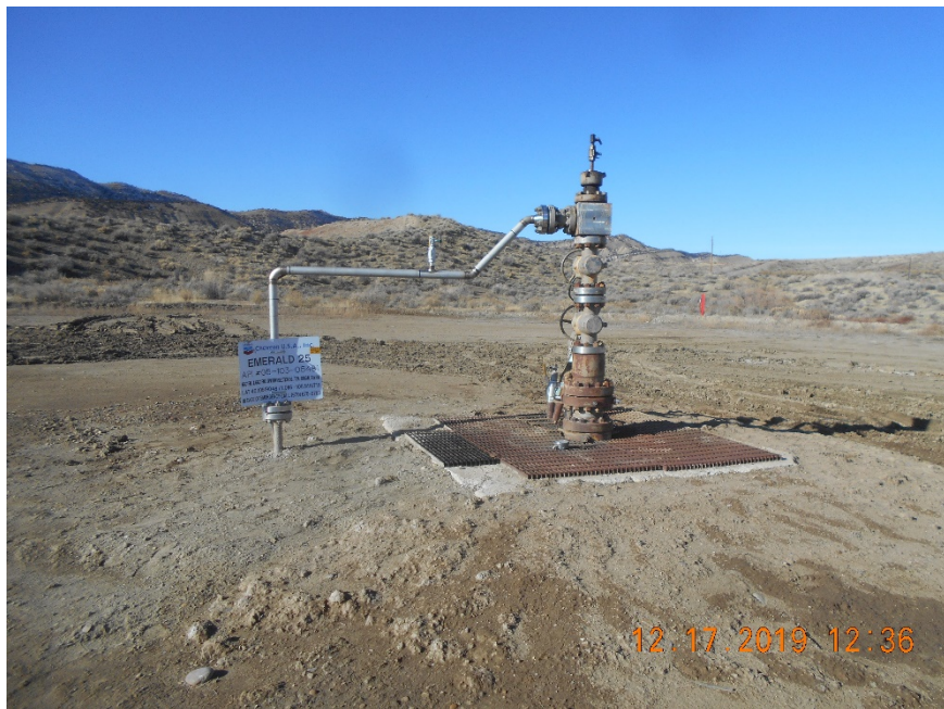
Injection wellhead.
