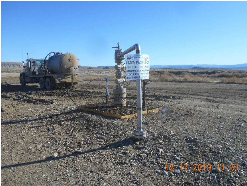
Injection wellhead.
