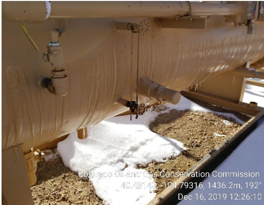
Photo 39: Sight glass removed, appears stained soil has been removed.
