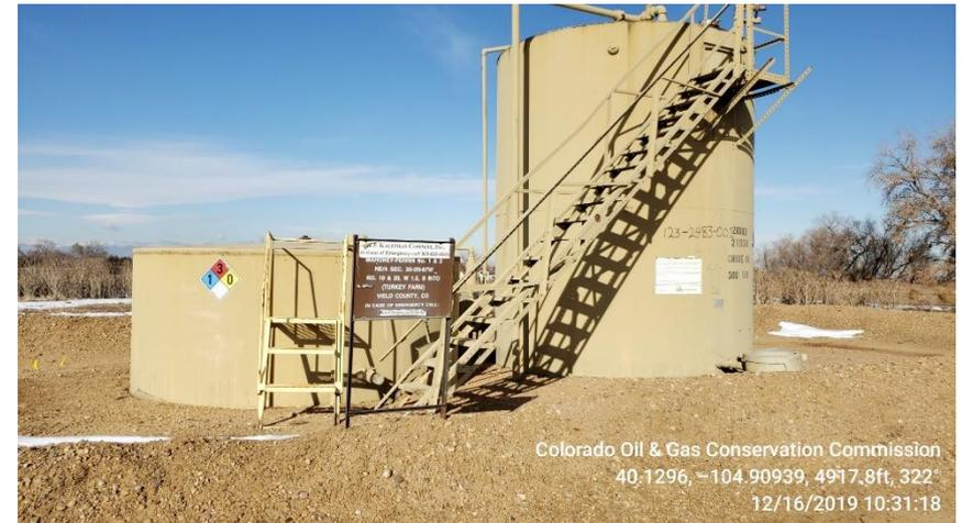
Photo 5 Stained soil at PU base appears to have been removed
