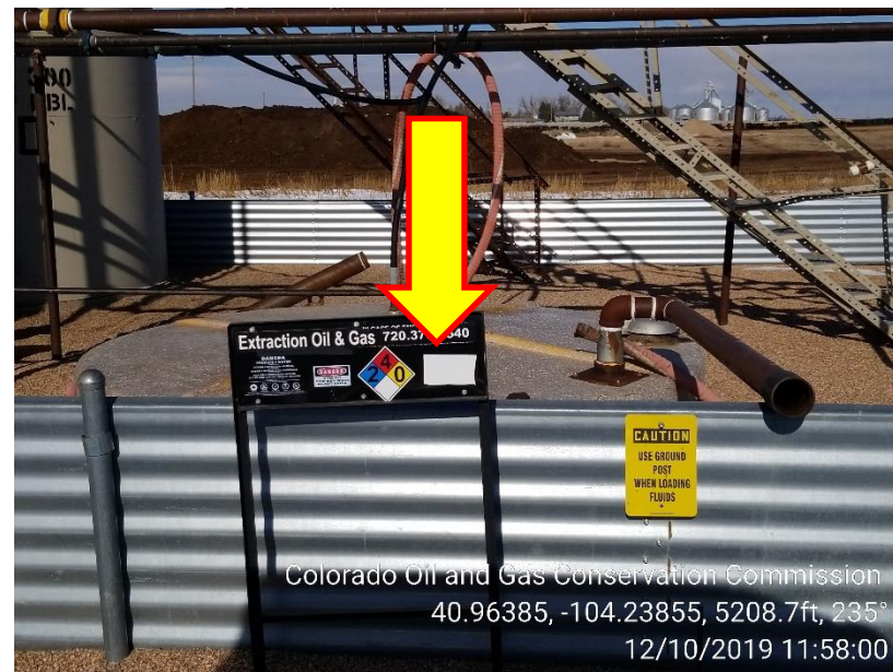
Photo 4 – Produced Water Tank - Capacity Label is missing
