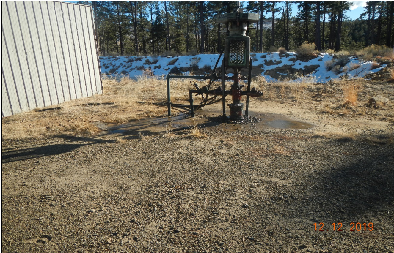
Photo 1. There is a constant flow of water coming from the wellhead.
