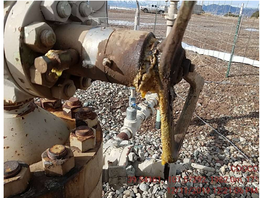
LEAKING FITTINGS PUMPER FIXED WHILE ONSITE
