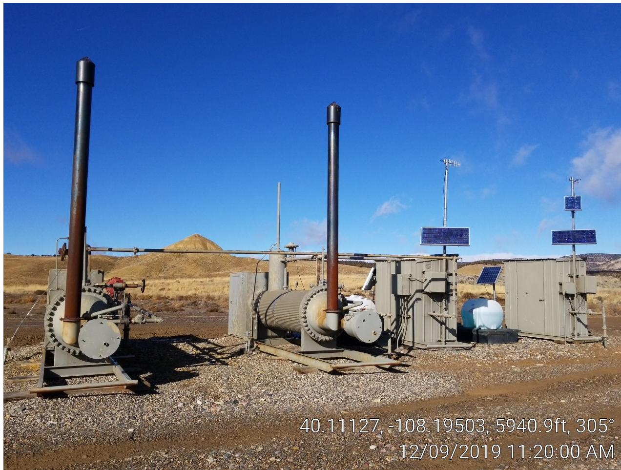
Photo 3. Separators & meter building.
