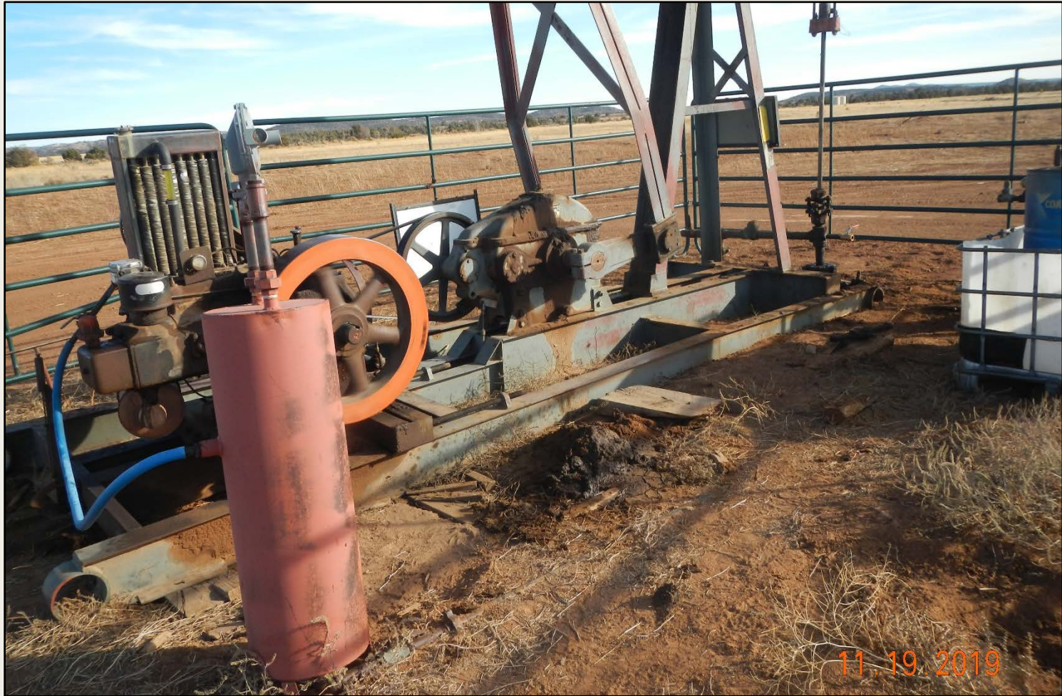
Photo 3. View of stained soils at well pump-jack, need to be cleaned and properly disposed of.
