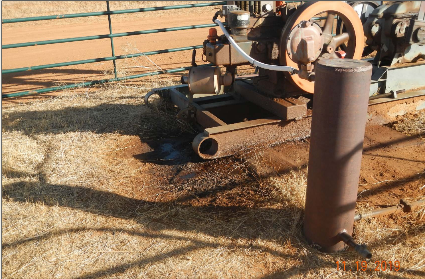
Photo 2. View of oily material and stained soils around pump jack.
