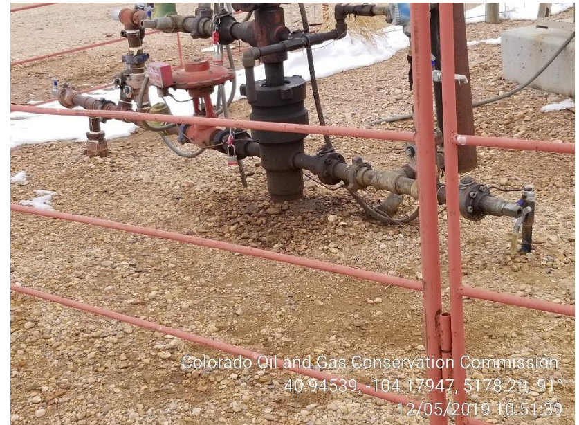
Photo 2 – Stained Soil at Wellhead
