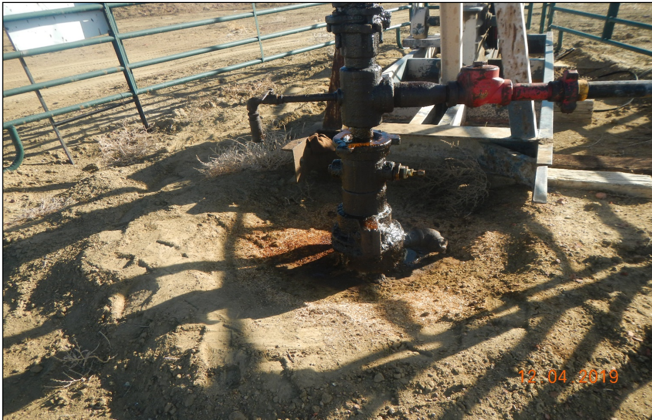
Photo 8. Oil leakage was observed from the wellhead.
