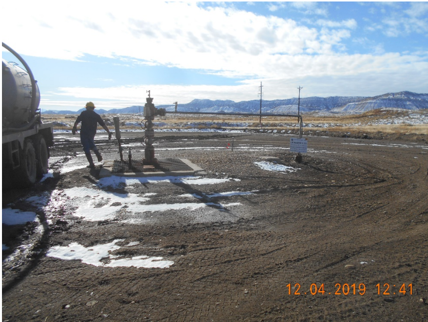
Injection wellhead
