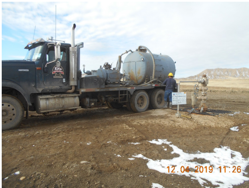
Injection wellhead.
