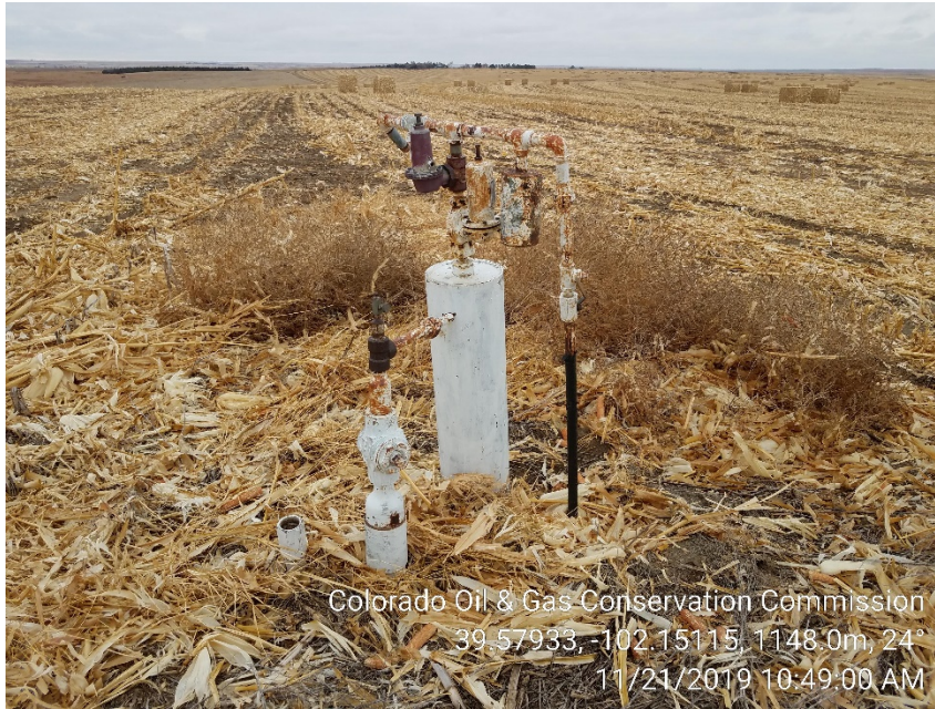
1. Wellhead and gas scrubber
