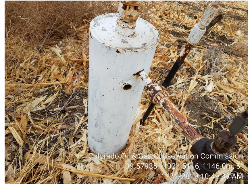
2. Gas scrubbers with broken 1" inlet line.
