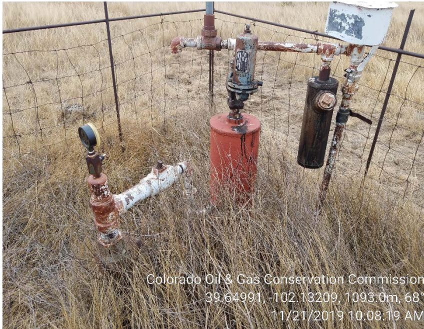
1. Wellhead and gas scrubbers
