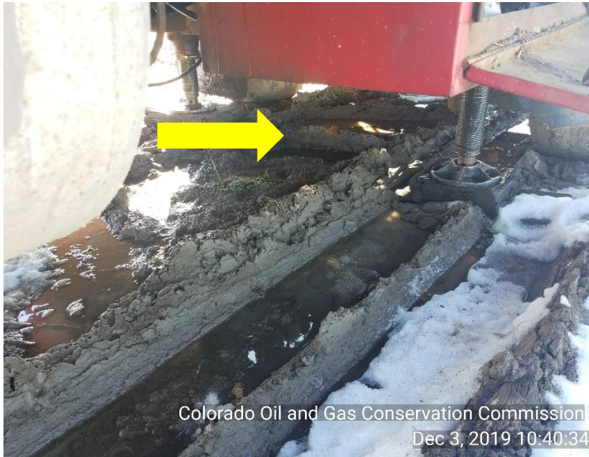
Photo 3 no secondary containment under rig, oil is dripping off motor and collecting on water and mud.
