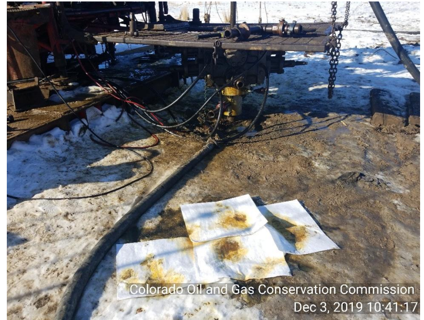
Photo 4 stained soil around well head.
