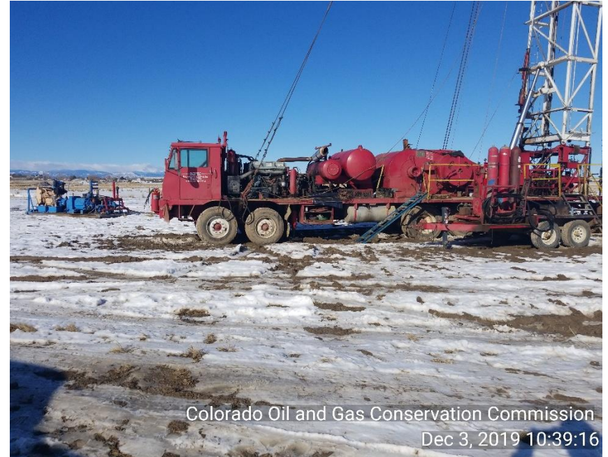
Photo 2 KPK rig not on secondary containment
