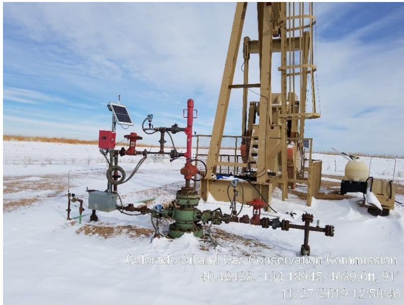
Photo 1 – Wellhead and Pumping Unit
