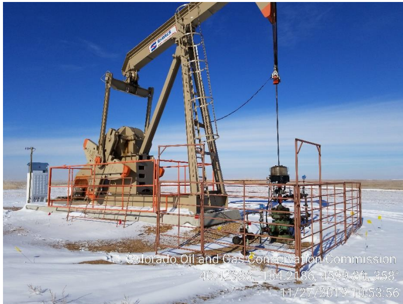
Photo 1 – Pumping Unit, wellhead sign Missing
