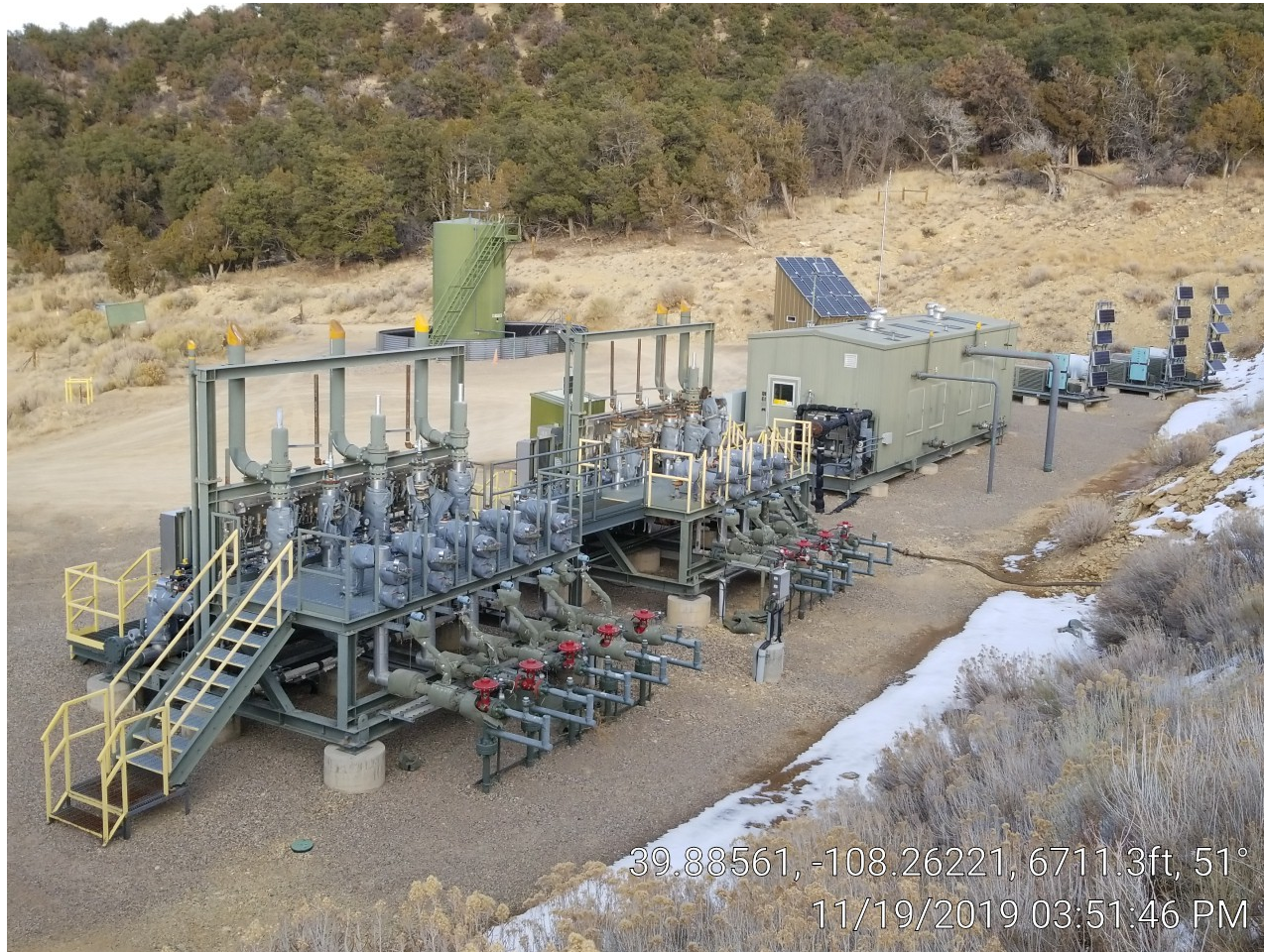
Photo 2. Battery, separator, chemical, and well header.
