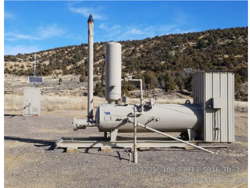
Photo 3. Separator & meter building.
