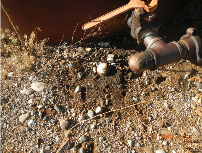
Photo 5. Stained soil at loadout valve.
