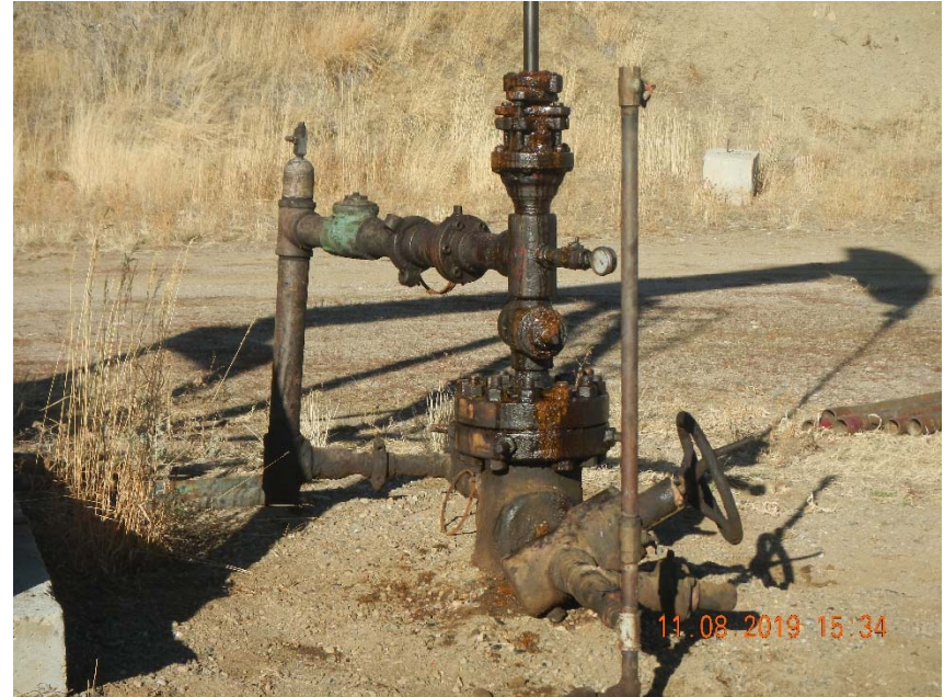
Photo 4. Stained soil at wellhead.
