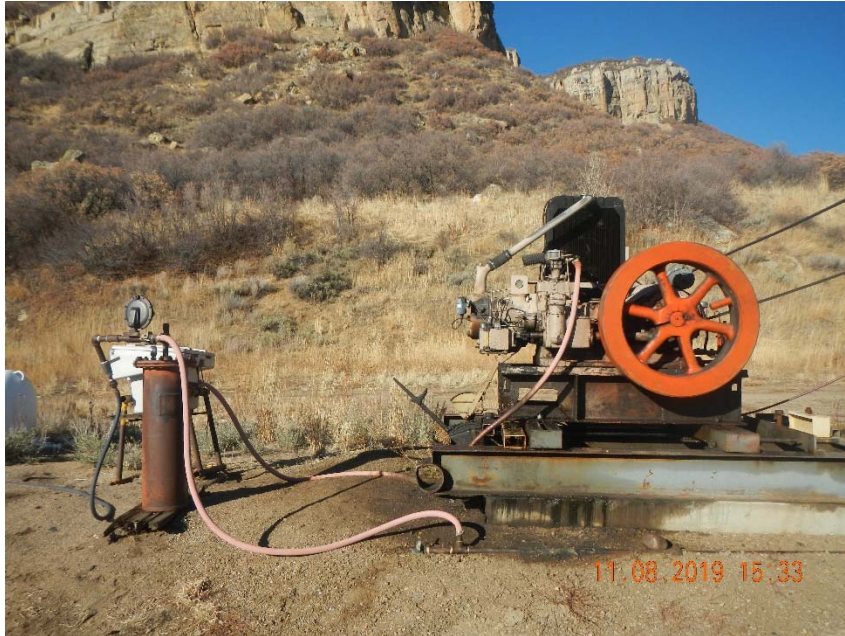
Photo 3. Stained soil at pump jack base.
