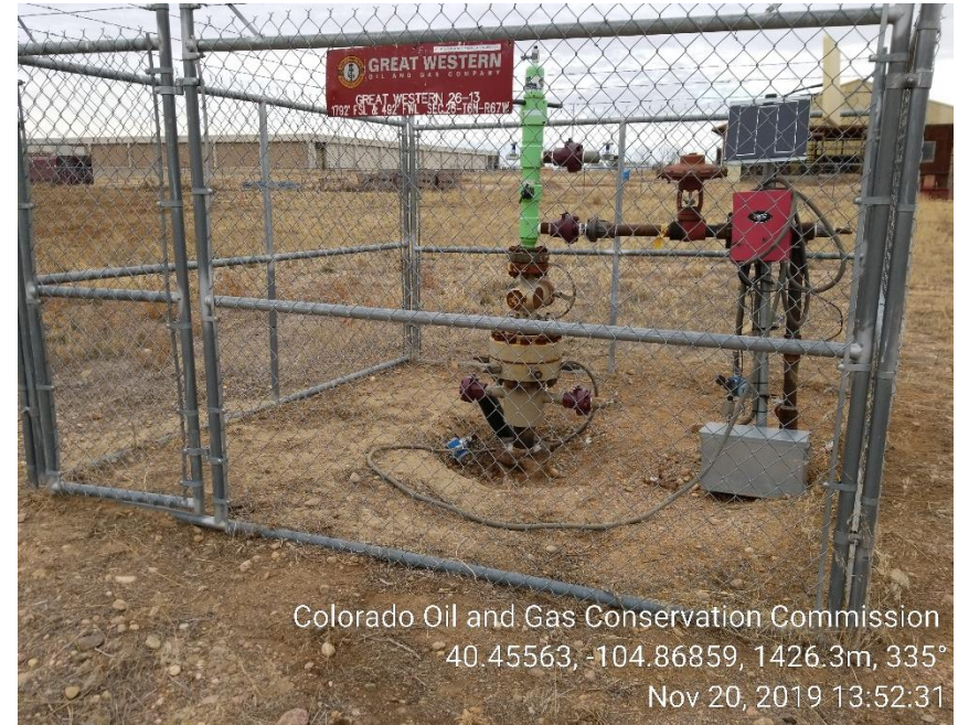
Photo 2: Wellhead; weeds removed
