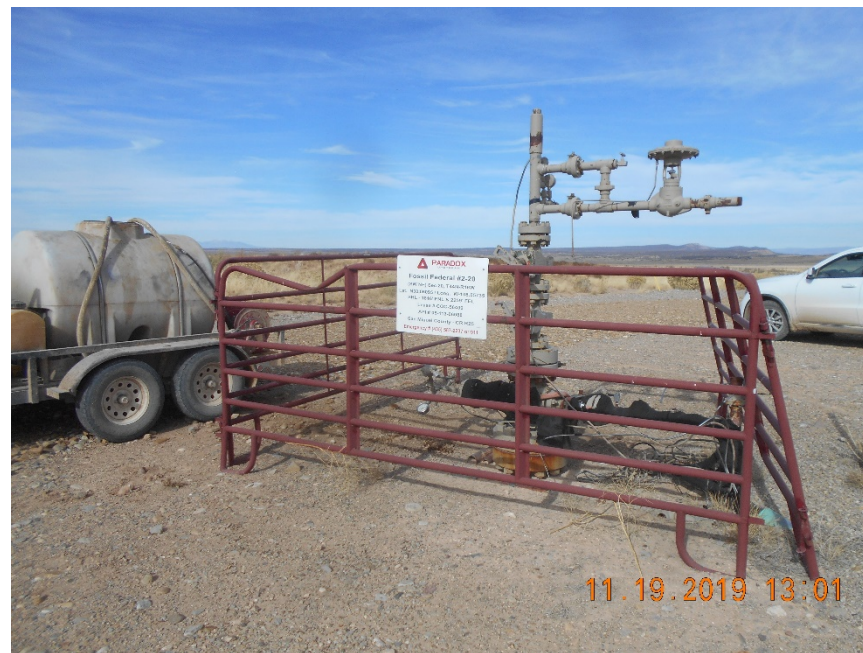
Temporarily Abandoned Wellhead with fence with sign.
