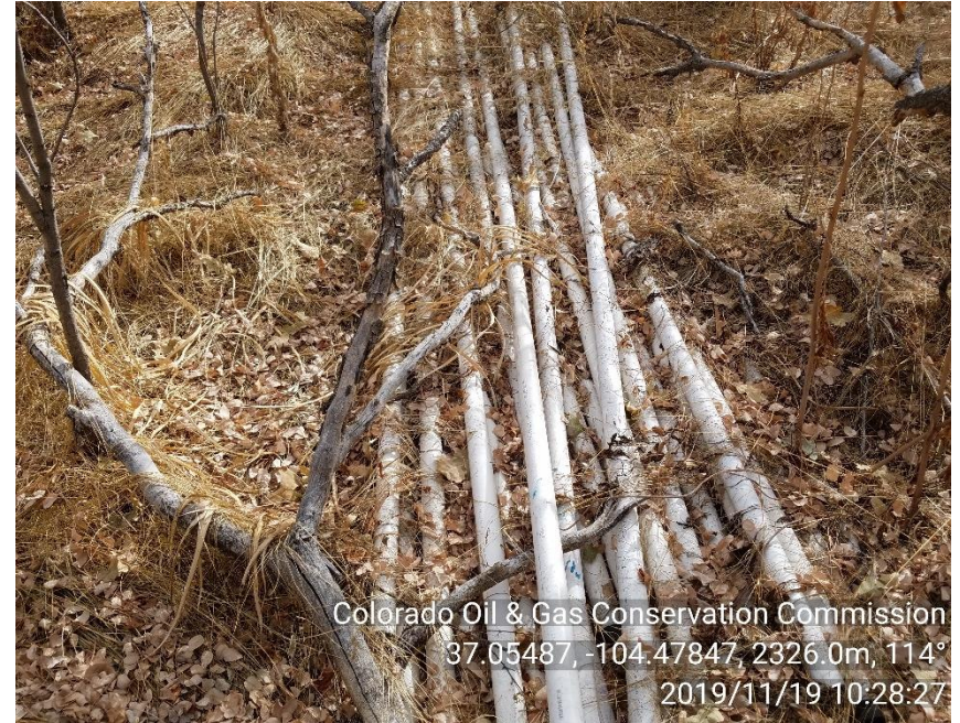
PHOTO 2: UNUSED EQUIPMENT LEFT ON LOCATION ( SEVERAL JTS OF 1 ¾" PVC PIPE USED FOR P&A). REMOVE UNUSED EQUIPMENT FROM LOCATION AS PER RULE 603.f. CA DATE 12-20-19.
