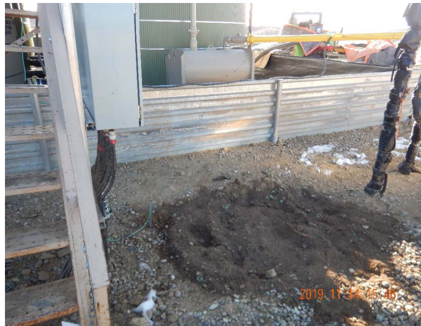
Photo #10 – Dark soil on north side of tank battery had hydrocarbon odor on inspection date.
