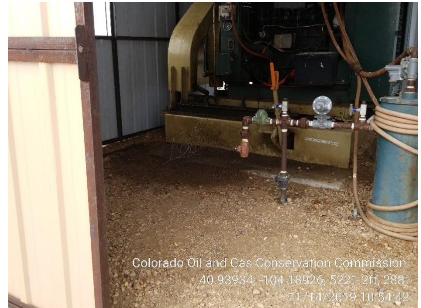
Photo 2 – Stained Soil at engine
